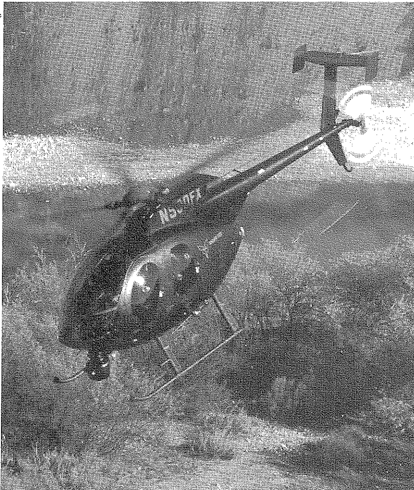
Typical of new equipment being developed for SOF is the McDonnell Douglas "Nightfox" helicopter shown here. Its infrared thermal imaging system permits night observation missions.
