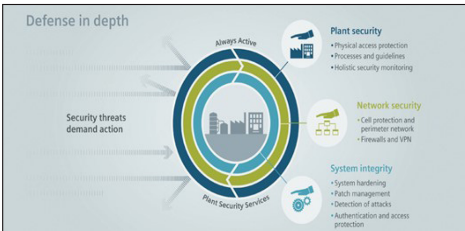
Figure 8-1. Defense-in-depth for ICS networks and the OT systems those networks support, with the Siemens SNOK IDS solution providing an early warning system for detecting attacks to strengthen system integrity 14
